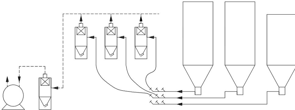
Central vacuum systems are used for the automatic transportation of granulated plastic resins to processing machines. One or several kinds of resins that may be stored in outside or in house silos, octabins, big bags, drying hoppers etc. can be supplied automatically. A proven modular system of the necessary components allows an improvement of the material flow for any kind of plastic production and can be customized to the special needs a certain process may request.
